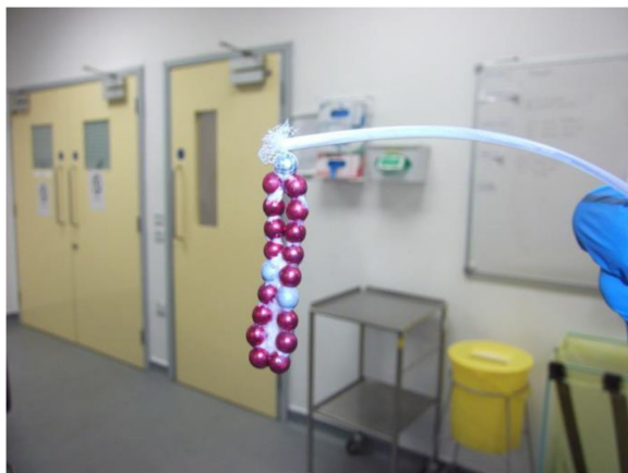
Fig. 6 Demonstration of the strong force upon which the basic magnetic retriever attaches to the ingested magnets
